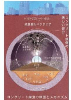
↑ (The causes and mechanisms behind concrete corrosion)
